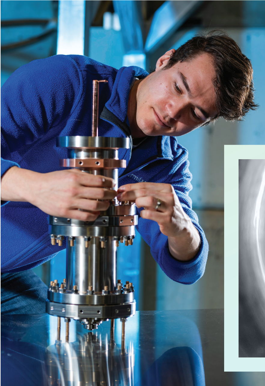
An IARC engineer assembles a radiofrequency power coupler for an industrial SRF accelerator
